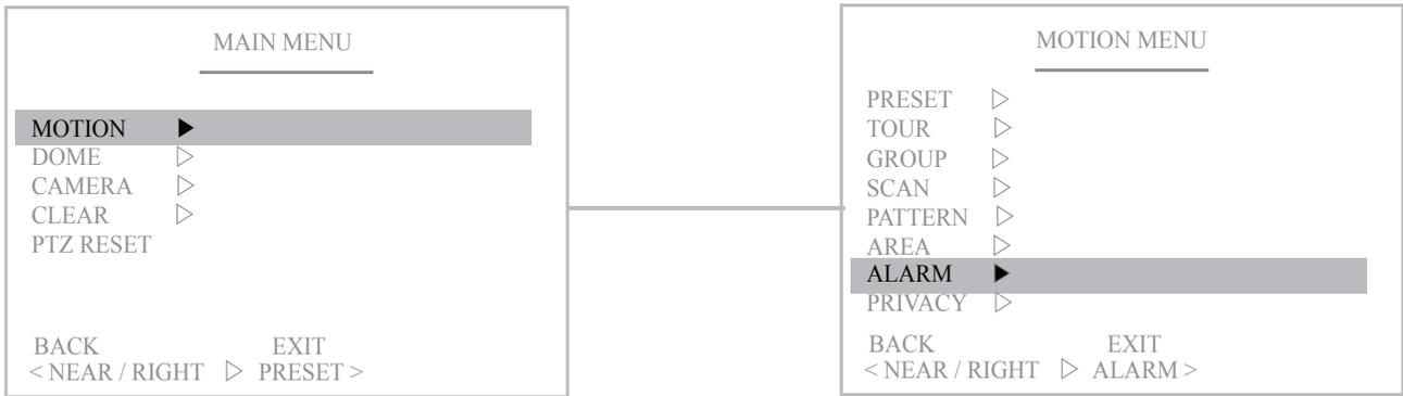
The Alarm function means that the camera moves to the programmed Preset position by the Alarm trigger. Maximum 8 Alarm functions are toured in order.
